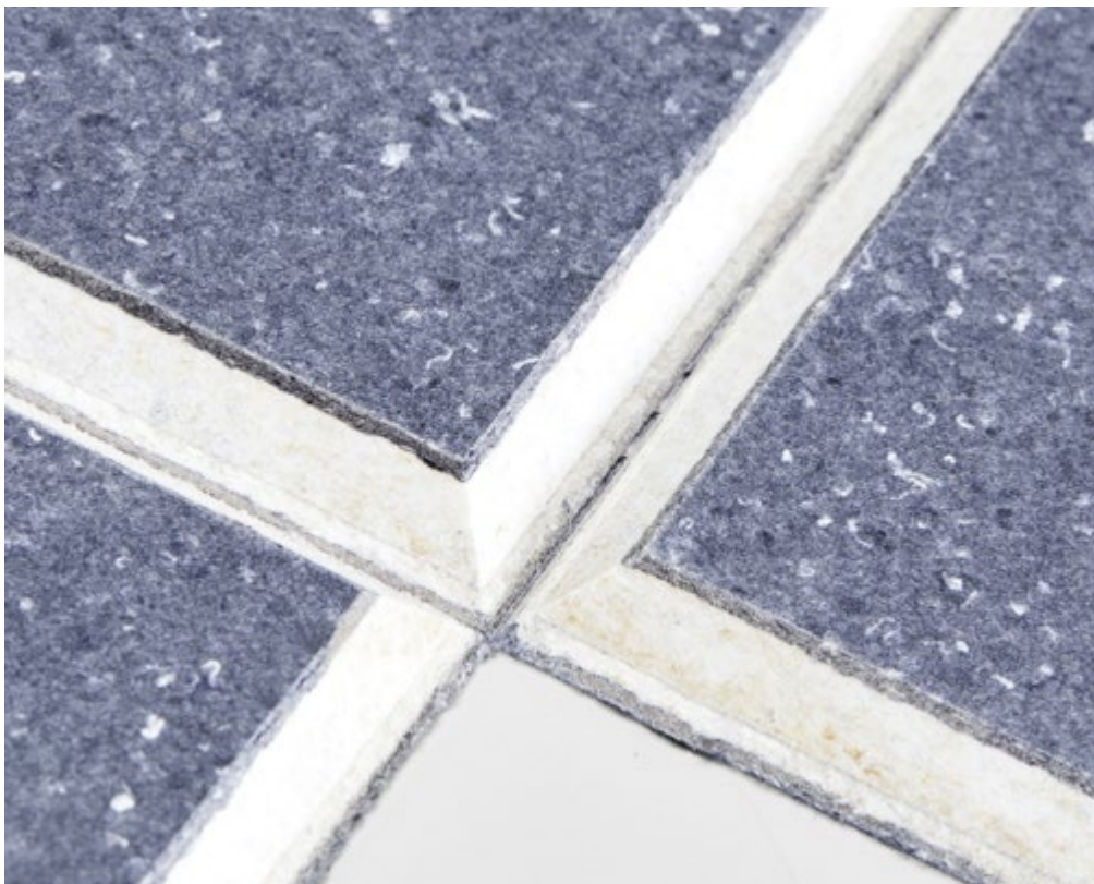
Miter-fold joint cut by a blade in a CNC machine
